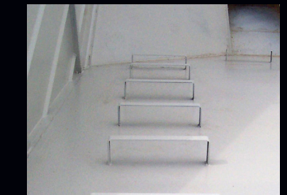
LADDER RUNGS Located on Inside of Trailer
