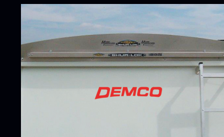
TARP CABLE RETURN Located on Front and Rear
