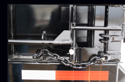
SAFETY DOOR OPENER The safety door opener is optional for the Latch closure
